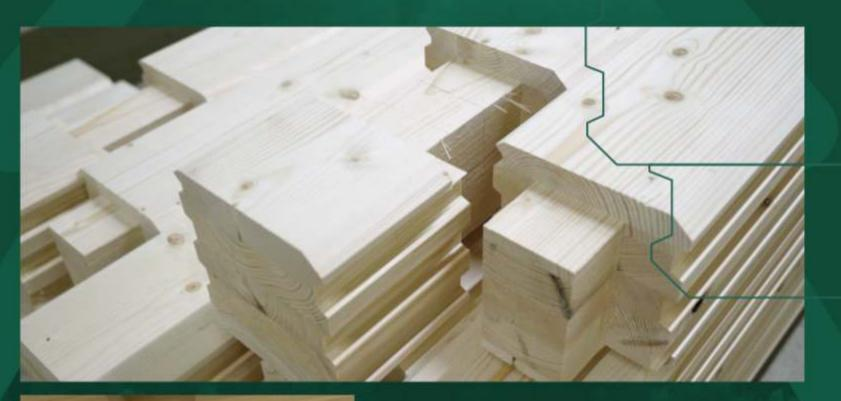
The timber is segmented into parts according to the specification. Saddle notches, holes, grooves, corner and assembly joints are cut
