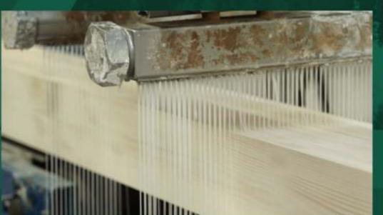
Joining lamellas up to 49 ft (~15 m) long using a hydraulic press
